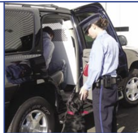
K9/Prisoner Transport Accommodates single prisoner on passenger side and K9 unit on driver side. Includes emergency exit door.
