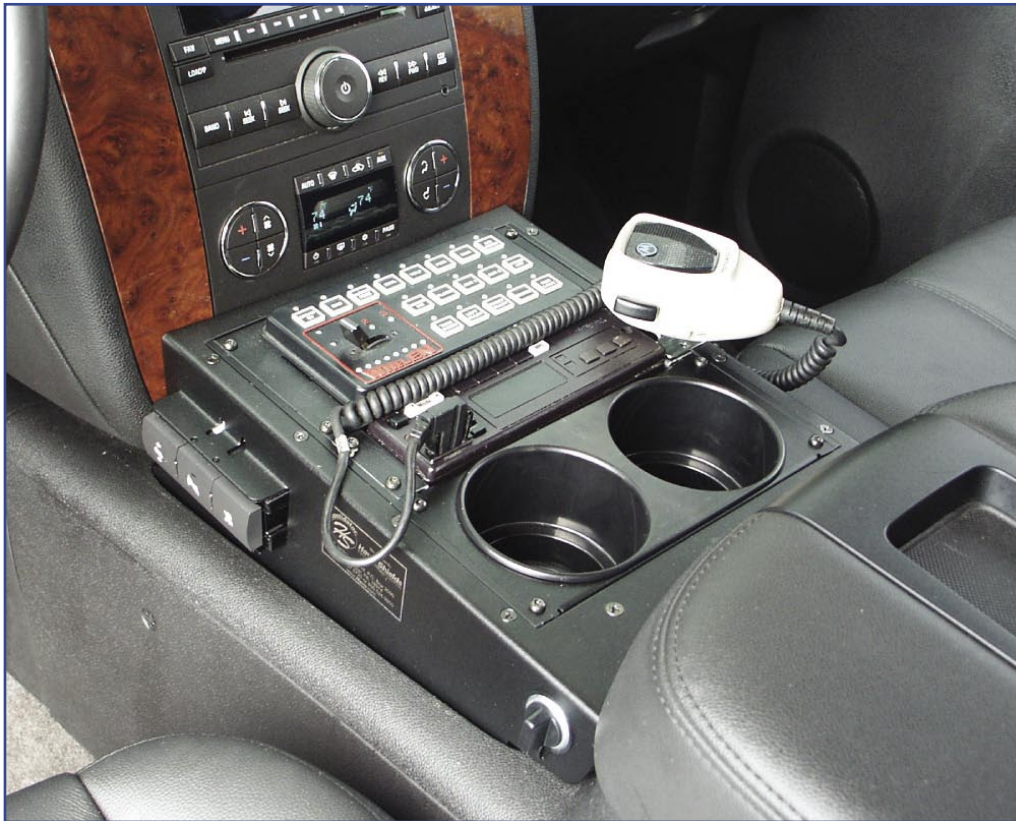
2007-2008 Chevrolet Tahoe Vehicle Specific Console This new vehicle-specific OEM replacement console provides professional and custom appearance without permanent modification. The console is manufactured from laser cut steel to precisely fit OEM trim. The formed steel housing and extruded aluminum frame provide strength for mounting up to 10" of emergency equipment. C-VS-1000-TAH
